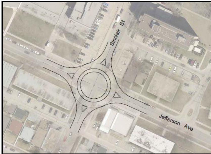
Figure 4: Modern Roundabout at Jefferson Avenue and Sinclair Street
