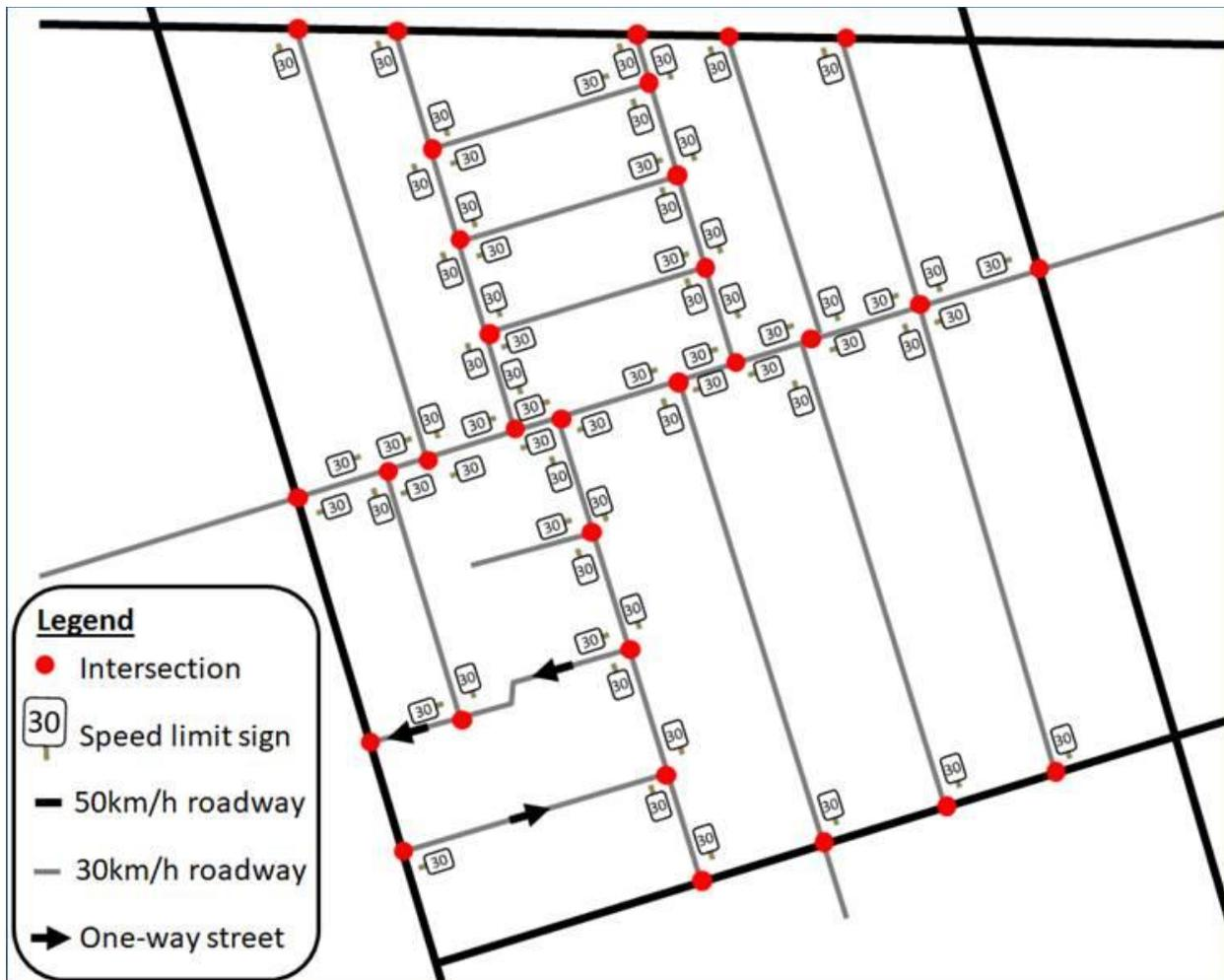
**Figure 2: Example of Reduced Residential Speed Limit Signage Requirements**
