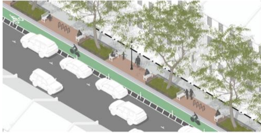
Long Planter Condition
