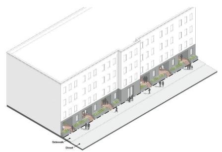
Figure 4 – Embedded Porch Frontage Design Elements
