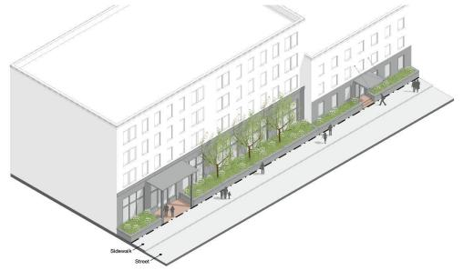
Figure 2 – Common Entry Frontage Design Elements
