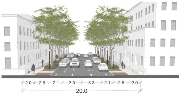
Figure 29 – Typical Framework Street Section
